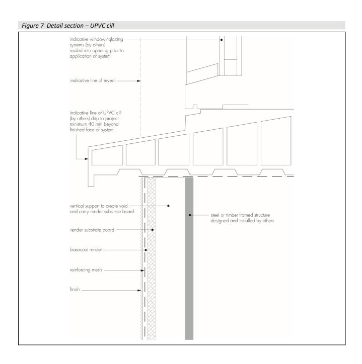
indicative window/glazing systems (by others) sealed into opening prior to application of system
