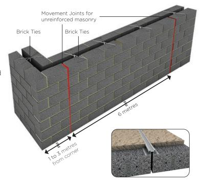
The adequate use of movement joints will help reduce stress build up in the substrate and thus reduce the risk of cracking. Movement joints must also be followed through the render.
